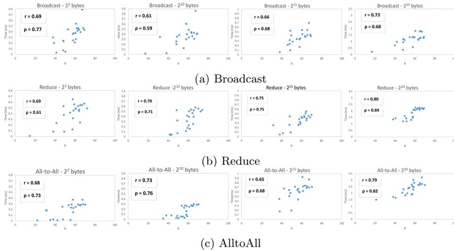
Fig. 4: The relation between background traffic ( $b$ ) and the average communication time of different collectives with different message sizes.
